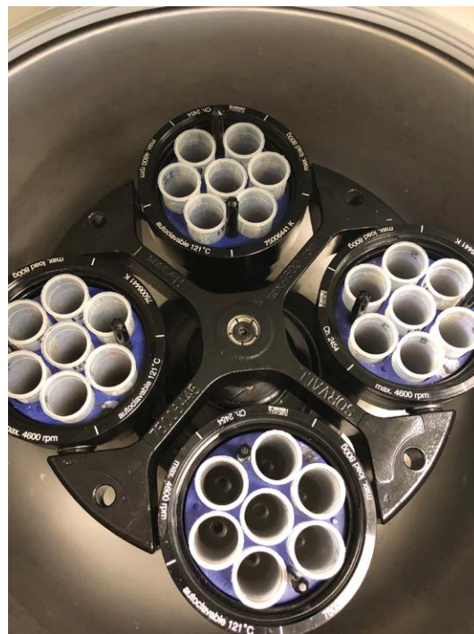
Fig. 4.6. An example of a centrifuge that contains a rotor holding four buckets and twenty-eight 50 ml tubes. Note that seven tubes are placed in a rack and then placed in the bucket. Each tube is numbered so that it corresponds to a specific sample.
