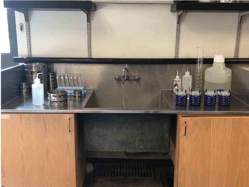
Fig. 4.7. A stainless-steel sink used for extracting nematodes from soil. Note that there is a set of small, medium and large sieves for wet sieving different types of nematodes. A bucket, a tray of twenty-eight 100 ml beakers and a wash bottle should be available for wet-sieving procedures. The sink has ample surface on both sides to perform wet sieving and prepare centrifugation.
