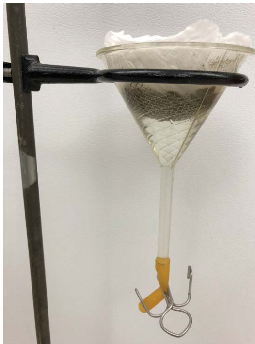
Fig. 5.15. A Baermann funnel set-up to extract nematodes from soil or plant tissue.
