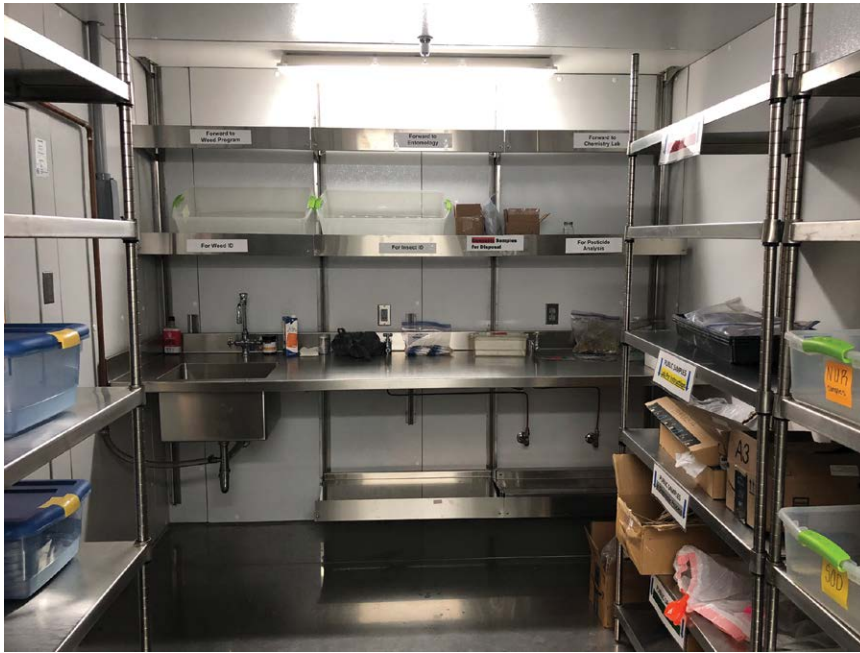
Fig. 4.2. An example of a walk-in cold room serving as a storage space for plant samples and temperature-sensitive laboratory materials. Note that multiple shelves offer better organization of samples in different diagnostic categories such as disease diagnosis, insect identification, weed identification and pesticide analysis.
