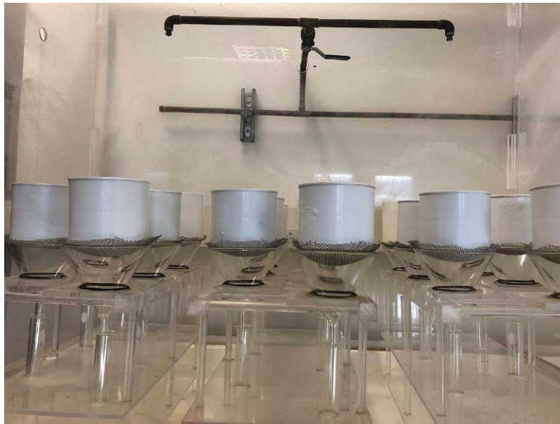
Fig. 4.8. An example of mist chamber used for nematode extraction from plant tissue. Note that each funnel is assembled from top to bottom: extension tube, paper layer, metal screen (for support), funnel and long glass tube. The extension tube is used only when a sample quantity is large and cannot be held on top of the funnel.
