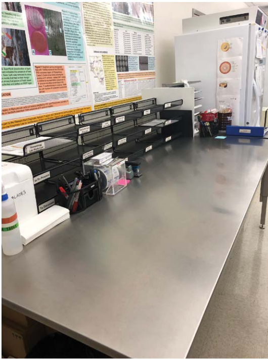
Fig. 4.1. A stainless-steel table serving a sample receiving and observation area. Note that a series of shelves are provided for better organization. This table can also serve as a dissection table, especially when a large plant needs to be cut to check for vascular discoloration or a tree sample needs to be examined for borer insects. A large table also makes sample photography easy (usually with a set of different-coloured boards used as backgrounds).
