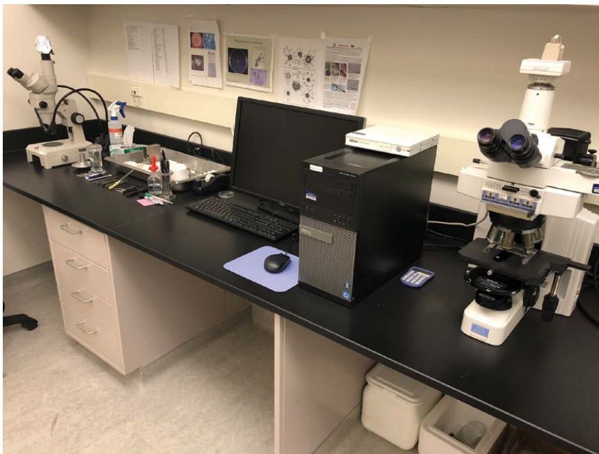
Fig. 4.3. An example of a setting for microscopic examination. Note that both dissecting microscope and compound microscope can be connected to a computer for image capture. Necessary supplies are in place to assist microscopic examinations.
